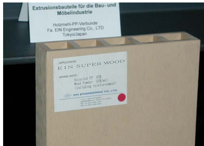
Wood Plastic Composite from Japan made from 55% (wt) wood powder and 45% recycled PP.
