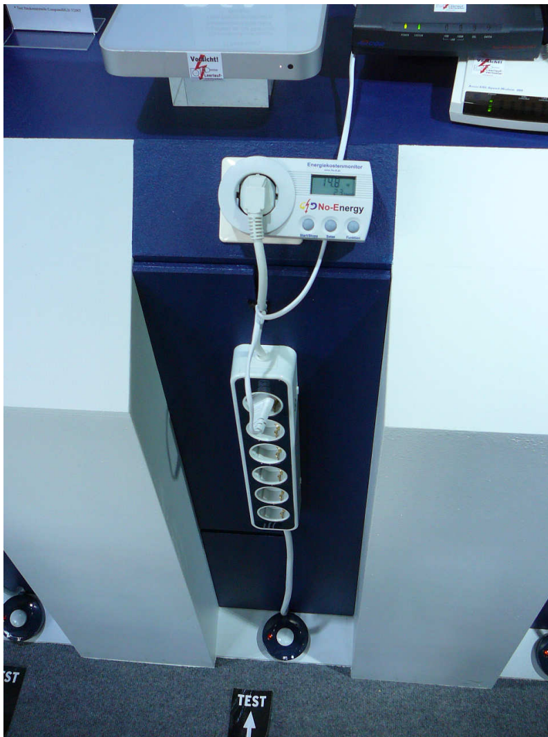
Picture 3 (left): With an energy cost monitor (“No-Energy”) office appliances can be checked for energy consumption in stand-by modus or even after disconnection. To avoid this waste you can use a multiple socket with can be comfortably switched off by foot switch (→ “TEST”), as being demonstrated at the Hannover Fair 2008.
