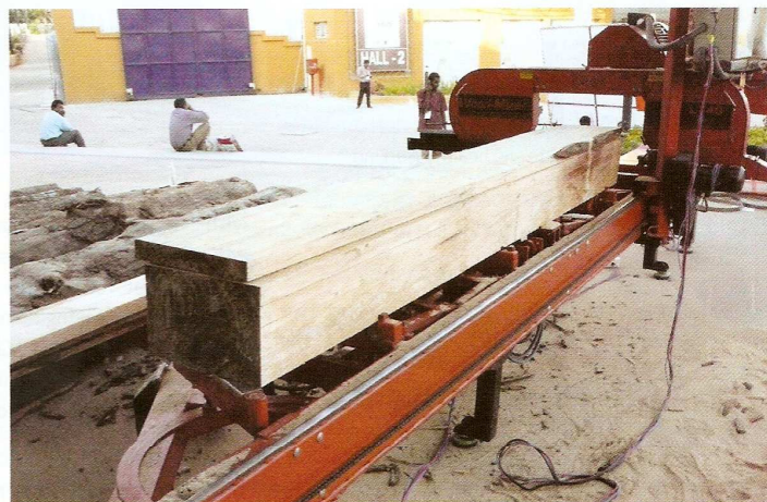
Portable sawmills, as presented here at Indiawood in Bangalore in March 2008, can help farmers to produce high quality timber for roof trusses and other construction elements from their agroforestry plantations and by this contribute to rural development.
